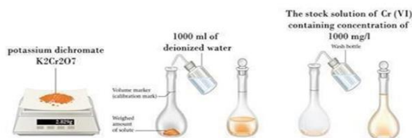
FIGURE 2. Preparation of Cr(VI) Stock Solution
